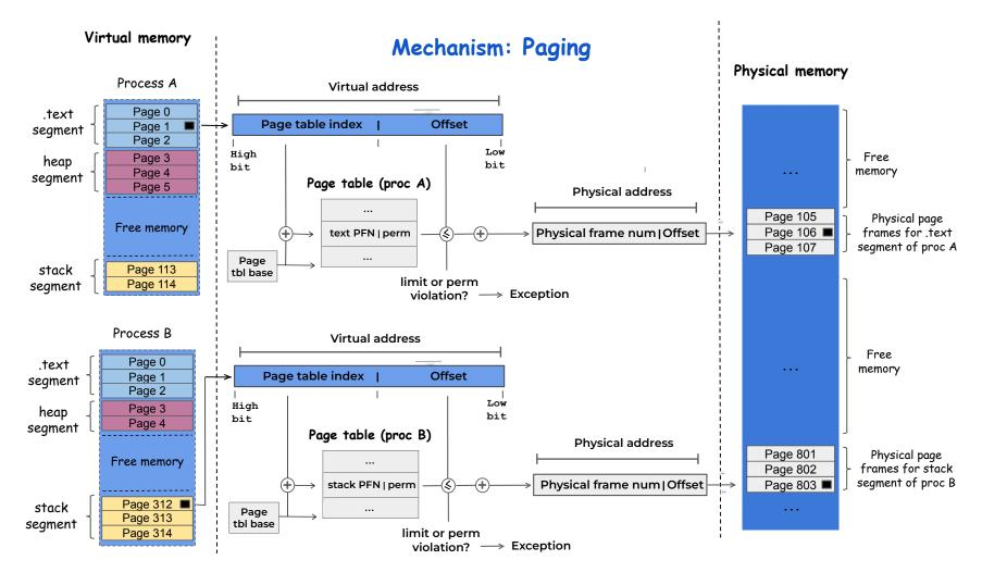
> Assume 32-bit virtual and physical address space, 20-bits for page table index and 4KB pages (i.e., 12 bits for offset)
