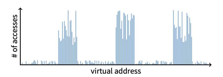
> A process can be in main memory iff all the pages it is currently using can be in main memory, by P. Denning (1968)
